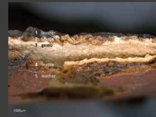
Profile view of the backing construction with different layers in detail.
