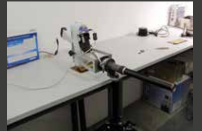
The analysis of the gold sheets by means of portable X-ray fluorescence. This fast and reliable analytical tool is specialized in distinguishing all kinds of metal alloys.
